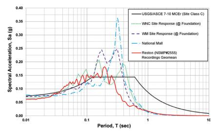
Figure 3. USGS MCE<sub>R</sub> for Washington, D.C., versus recorded/computed motion. Adapted from Wells et al.
