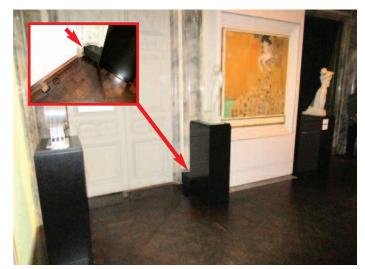
Figure 6. Enclosure (red arrow) constructed around vibration monitor in second-floor gallery.
