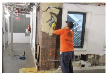
Figure 5. Dropping terracotta blocks with plaster finish from a height during vibration trials.
